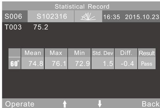
Figure 24 Single Angle Measurement in Statistical Mode
