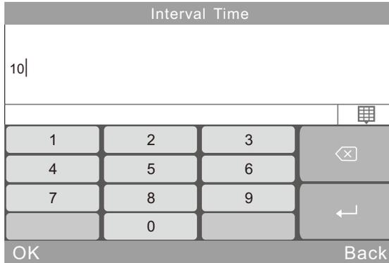
Figure 37 Interval Time Setting in Continuous Mode
