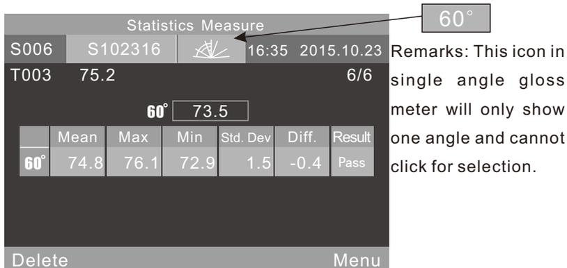
Figure 11 Single Angle Measurement under Statistical Mode
